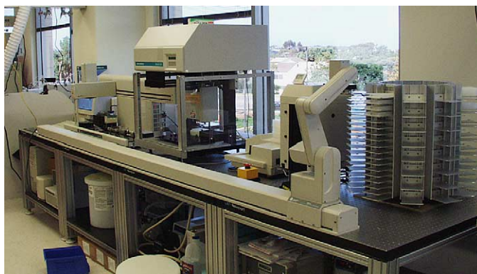
Fig. 1. SAGIAN™ core robotics system supporting in vitro ADME assays.
